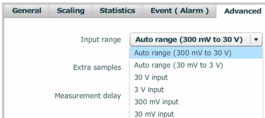
Figure 7 Selecting Voltages up to 30 V
