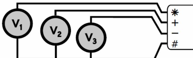
Figure 10 Wiring for Single Ended inputs
